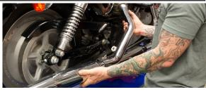
. Remove pulley cover and front exhaust pipe.
