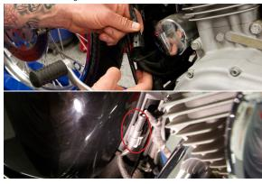
Loosen heat shield clamps and remove heat shields from both the front and rear head pipes.
