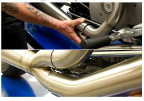
Install and tighten muffler mounting flange bolts 5/16"x 3/4".
