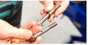
Install one o-ring onto each end of the oil-channel spacer.
