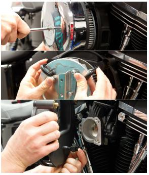
Remove plug from back of OEM backing plate and zip-tie out of way.
