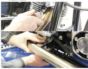
Install front 02 sensor (this has the grey plug on the end of the sensor wire) use supplied adaptors for 12mm 02 sensors.
