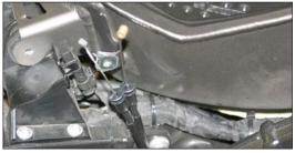
Remove muffler mounting bolt and inside spacer, these will not be re-used.
