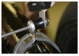
27. Align muffler and securely tighten the x-ring bolts in a cross pattern.
