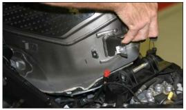
Remove both cables from servo carefully. Do not turn servo, the servo must stay plugged in and on motorcycle.
