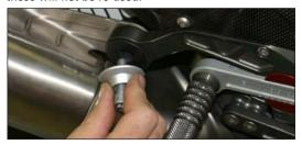
Loosen joint clamp and remove muffler assembly.
