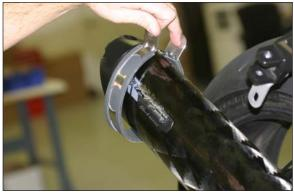
26. Loosely attach to bracket using the supplied bolt with decorated washer and spacer using the supplied 8mm flange nut.
