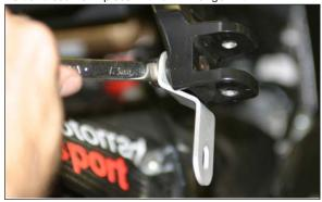
24. Attach TBR muffler to supplied slip-on tube using the provided four 6x20mm socket head cap screws, washers and thread-lock.
