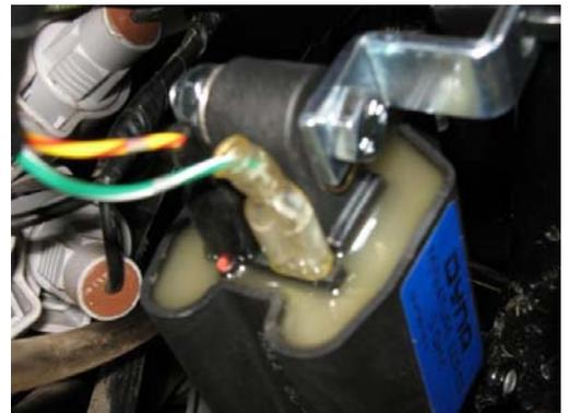
8. Front coil wires connected.
