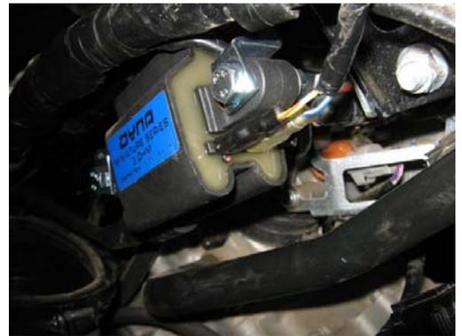
4. Rear coil wires connected.
