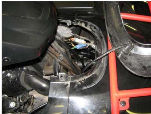
5. Remove panel under handlebars to access front coil wires.
