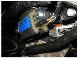
4. Rear coil wires connected.
