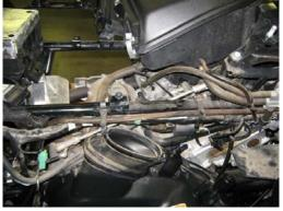
1. Disassembly required to access rear coil.
