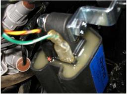
8. Front coil wires connected.
