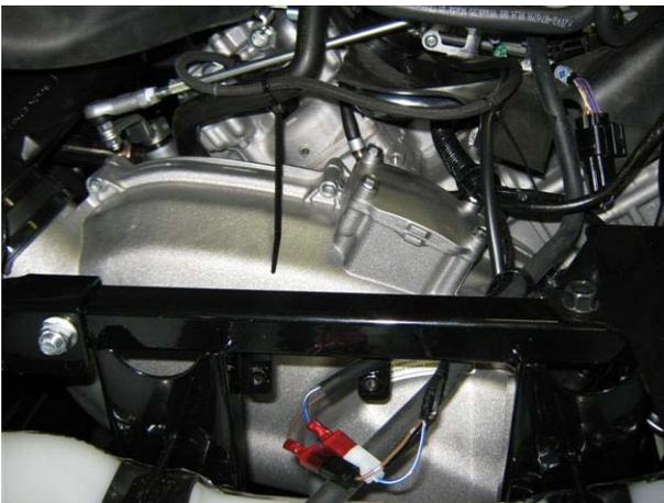
Step 7, 8: Wire routing. (Rear Cylinder)
