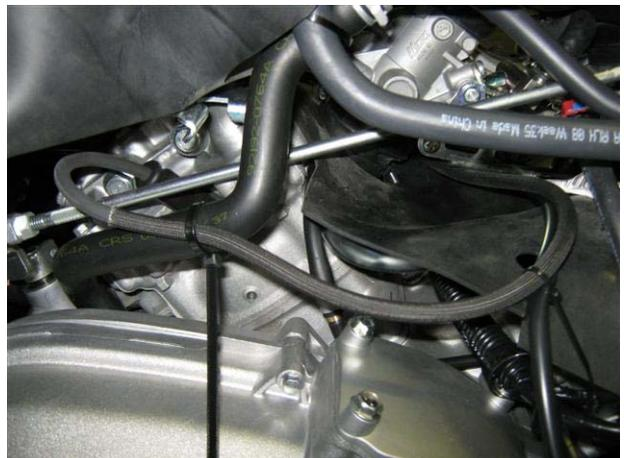
Step 8: Wire routing. (Rear Cylinder)
