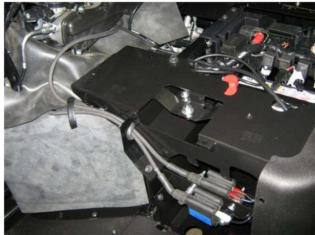
Step 7: Wire routing. (Front Cylinder)
