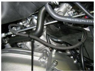
Step 8: Wire routing. (Rear Cylinder)
