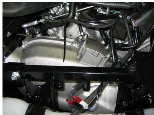
Step 7, 8: Wire routing. (Rear Cylinder)
