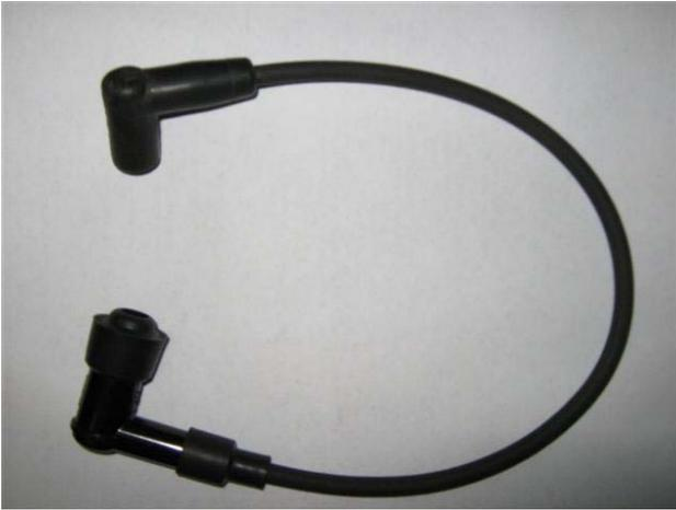
Step 3, 8: Attach spark plug cap to wire.
