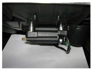
Step 6: Attach coil primary wires
