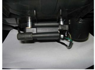
Step 8: Attach spark plug wire
