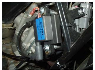
Step 4: Mount Dyna coil with long bolts and spacers.
