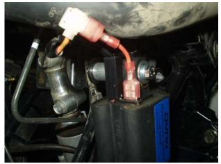
Step 6: Connect Orange to Orange to coil without dot.
