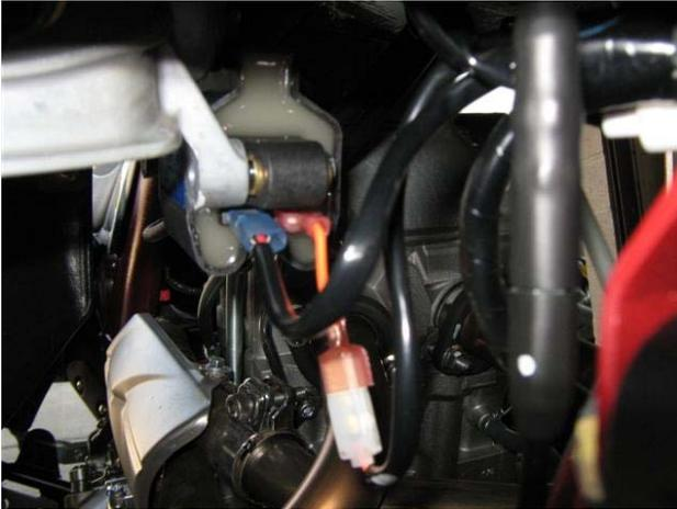
Step 3: Attach coil primary wires.
