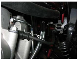
Step 2: Screw original spark plug cap onto wire. Press secondary wire onto coil and spark plug.
