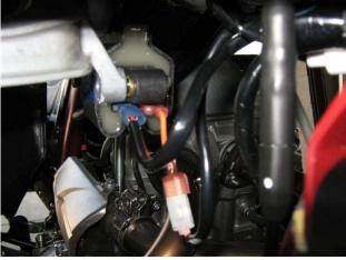
Step 3: Attach coil primary wires.
