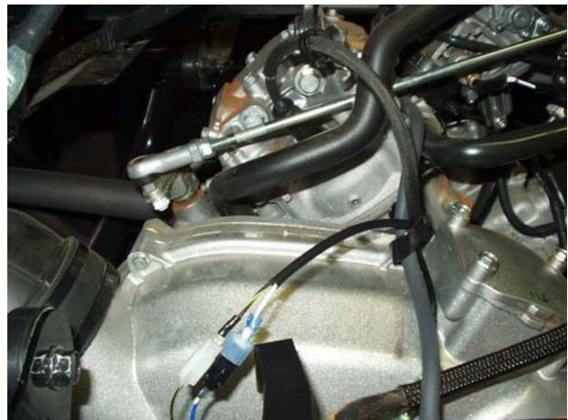
Step 8: Wire routing. (Rear Cylinder)
