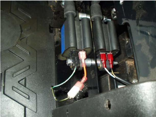
Step 6: Attach coil primary wires.
