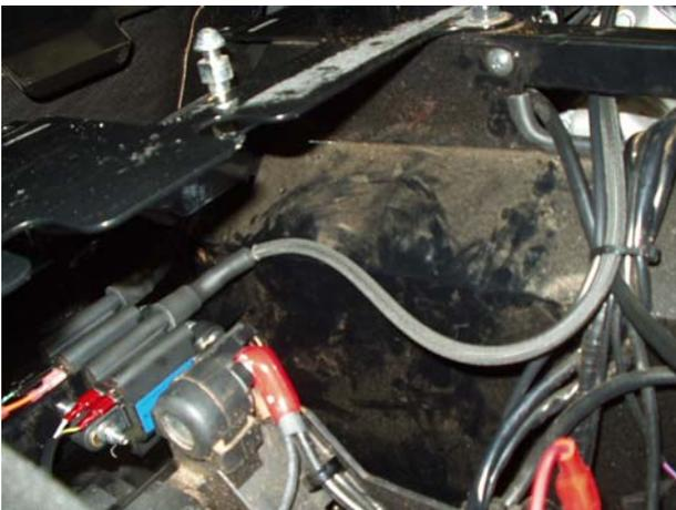
Step 7: Wire routing. (Rear Cylinder)
