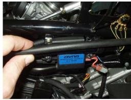
4. Dyna coil for rear cylinder, mounted to frame.
