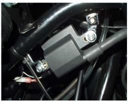
2. Dyna coil for front cylinder, mounted to frame.
