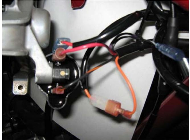
Picture7: Coil connections to Dynatek Coil(1)
