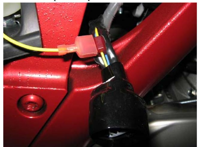
Picture6: Coil connections to stock ignition coil.
