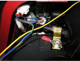
Picture3: Expose the Yellow TPS signal wire.
