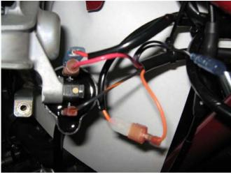
Picture7: Coil connections to Dynatek Coil(1) Picture8: Coil connections to Dynatek Coil(2)
