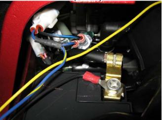
Picture3: Expose the Yellow TPS signal wire.
