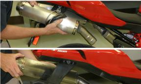
Install Two Brothers Racing V.A.L.E<sup>™</sup> slip-on system. Attach the left side slip-on tube to the left muffler and right side slip-on tube (the straighter and shorter slip-tube) to the right muffler, using the 8 (eight) 6x14mm socket head cap screws and split lock washers provided. Keep loose for now.
