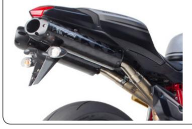
Align mufflers and tighten the 6x14mm V.A.L.E.<sup>™</sup> hardware when the slip-on tube clearance and the muffler alignment is correct. It may be easier to tighten one bolt first, then remove the slip-on tube assembly to tighten all of the rest of the hardware.
