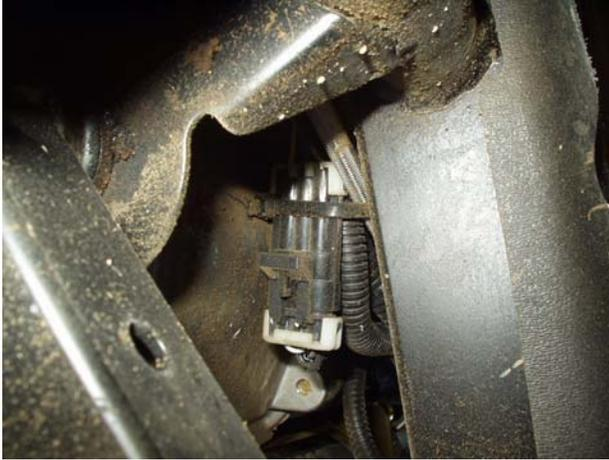
**Picture 2: Throttle Position Sensor connector**
