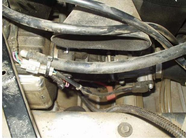
**Picture 3: Injector connectors with Intercepts**
