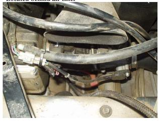
Picture 3: Injector connectors with Intercepts Located behind rear service panel
