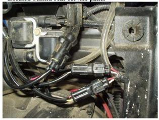
Picture 4: Ignition Coil Located behind rear service panel
