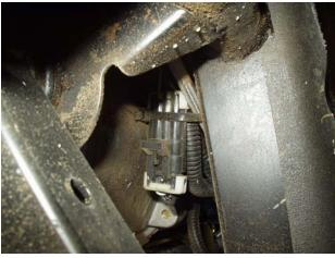
Picture 2: Throttle Position Sensor connector Located behind air filter
