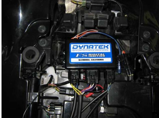
**Picture 3: Crankshaft Position Sensor connection
