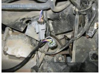
Picture 3: Ground connection Located right of the battery
