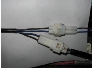
Picture 1: Crankshaft Position Sensor connection Located left of the battery
