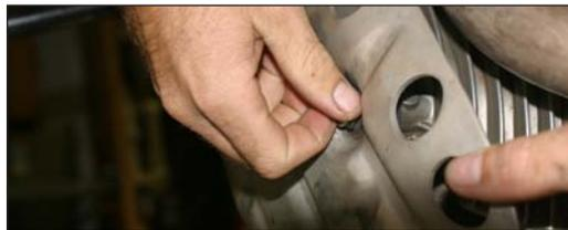
3. Remove OEM muffler assembly.
