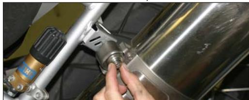
4. Remove both O2 sensors from head-pipe.
