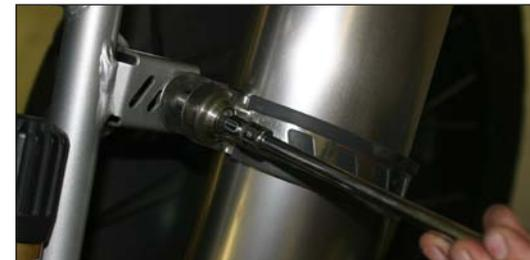
13. Check alignment and tighten X-Ring bolts, then muffler clamp bolt and finally barrel clamp.
