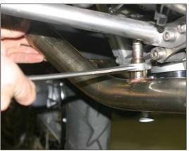
10. Attach TBR muffler to supplied slip-on tube using the X-Ring and 4 socket head cap screws with provided lock washers, leave loose for now.
