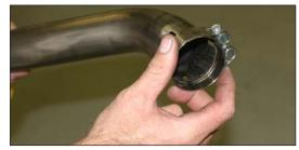
12. Slide rubber lined muffler clamp over muffler and install onto motorcycle using the OEM decorative washer and supplied bolt, leave loose for now.
