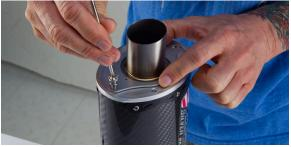
Place new carbon fiber cap onto muffler assembly. Attach by evenly 5. tightening the remaining four torx screws.
