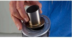
4. Install retaining ring using two of the supplied stainless steel torx screws. Align tallest point on the powertip with the top of muffler. After alignment is confirmed proceed to tighten torx screws.
