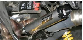
5. Align muffler and tighten the 4 X-Ring bolts.
