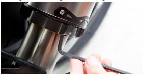
6. Tighten barrel clamp.
