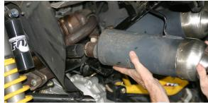
Attach TBR slip tube to TBR muffler using the 2 piece X-Rings and 6x20mm socket head cap screws with lock washer that are provided. Leave loose enough to make some adjustments on the UTV.
