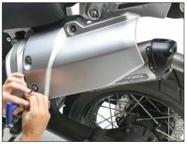
Before you run the bike, clean off all fingerprints and dirt, as any oily residue will etch the metal and become somewhat permanent when the system gets hot. Also, remove any protective plastic from the name badges on the muffler canister(s) or the muffler clamp(s). Run the bike and enjoy. It is normal for some white smoke to appear the first time you start the bike. This is packing/manufacturing oil from inside the pipe burning off. After 50 to 100 miles, recheck all fasteners for tightness.
