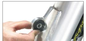
Attach slip-on tube to TBR muffler using the provided 4 6x20mm bolts and lock washers with X-ring. Leave loose for now.
