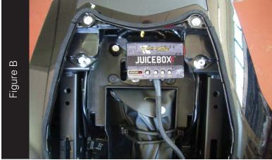
3. Using the supplied velcro, secure the Juice Box Pro in the tail section as shown in Figure B.
