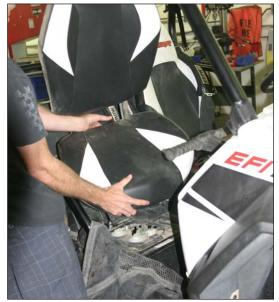
3. Tilt the panel forward behind the seats to access the header pipes.
