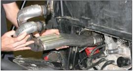
Remove muffler retaining springs(2) and remove OEM muffler assembly.
