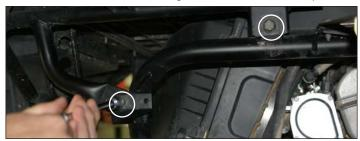
8. Install new supplied mounting bracket in both wheel wells using supplied 8x25mm bolts and rear bolts will use supplied 8mm nuts.
