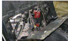
Remove exhaust pipe joint springs(2) above rear right wheel
