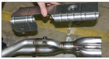
Attach the hanger bracket to the TBR center muffler using the 4 (four) 6x14mm socket head cap screws and split lock washers provided.
