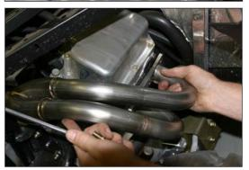
9. Locate slip-fit joint exhaust pipes and attach with supplied springs right side slip tube marked "R" to triple collector marked "R" and the same with "L" to "L" and "C" to "C". The left side exhaust pipe uses OEM tension stop(remove from OEM exhaust and install on TBR.
