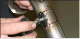
Mount supplied muffler mounting brackets to bed support using the supplied 8x35mm socket head cap screws and lock washers provided, leave loose for now.
