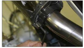
9. Secure muffler assembly mid-pipe and hanger bracket bolts. Tighten securely.
