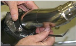
7. Insert slip tube of V.A.L.E.™ muffler assembly into OEM head pipe. Loosely install supplied 8x35mm hanger bracket bolt and 8x16mm slip-tube bolt.
