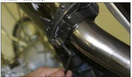
Secure muffler assembly mid-pipe and hanger bracket bolts. Tighten securely.
