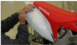
3. Remove lower OEM muffler mounting bolt.
