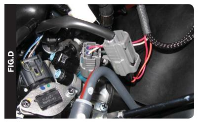
5. Attach the Juice Box Pro harness to the stock wiring harness and the fuel injector as shown in Figure D.
