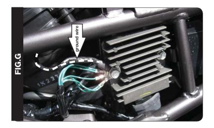
11. Attach the ground wire from the Juice Box Pro to the common ground location at the regulator/rectifier as shown in Figure G.
