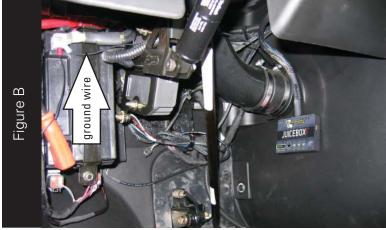
3. Using the supplied velcro, secure the Juice Box Pro to the driver side engine cover as shown in Figure B.
