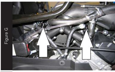
12. Locate the fuel injectors above the engine as shown in Figure G.
