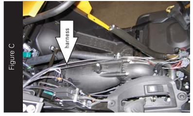
5. Route the Juice Box Pro harness over the engine cover and route the harness along the intake plenum as shown in Figure C.
