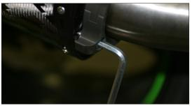
10. Tighten barrel clamp.
