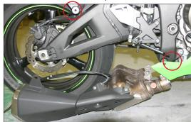
6. Attach TBR muffler to slip-on tube using the 4 6x20mm S.H.C.S. and lock washers provided. Leave loose for now.
