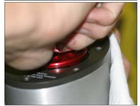
10. Re-install P-tip (with spark arrestor if applicable). Install Larger wave-washer on top of the P-tip if you are not using spark arrestor. There always needs to be 2 pieces under the endcap whether it is p-tip and washer, p-tip and spark arrestor, spark arrestor and washer, or none at all. See Diagram.
