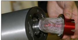
3. Loosen M2R retaining nut with the core nut tool that came with your original exhaust system, uses a 27mm socket.
