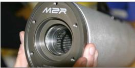
Remove old packing material, may be easier with pliers. Install new packing material, the cutout section of the packing is the top, so that it slides under the hanger bracket.
