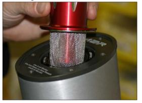
11. Align P-tip so that the slant is facing up. Re-install endcap and torx bolts, tighten in a cross pattern.
