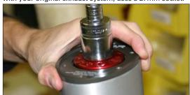
Remove outlet, may require use of a rubber mallot if tight, hitting the edge of the outlet in the direction of exhaust flow. You may also use the M2R outlet removal tool (purchased seperately part # 005-99-T175).
