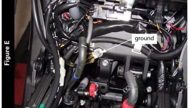
Attach the ground wire from the Juice Box Pro to the common stock ground wire location as shown in Figure E.
