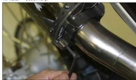
Using the OEM bolts, secure muffler assembly mid-pipe and hanger bracket bolts. Tighten securely.
