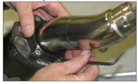
Insert slip tube of V.A.L.E.™ muffler assembly into OEM head pipe. Loosely install hanger bracket OEM bolt and OEM slip-tube bolt.  Securely tighten the 4 (four) 6x20mm hex head bolts of the V.A.L.E.™ assembly.
