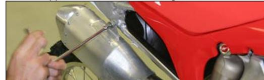
5. Remove OEM muffler assembly. Remove OEM header, save header nuts for later use.
