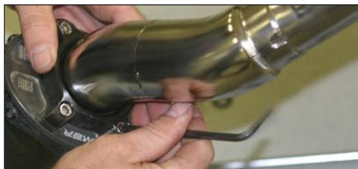
7. Install TBR header using OEM nuts.
