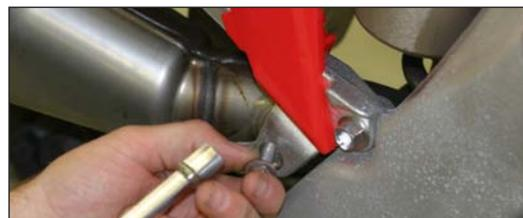
4. Remove upper OEM muffler mounting bolt. Retain for use.
