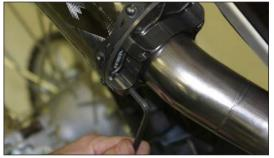
10. Using the OEM bolts, secure muffler assembly mid-pipe and hanger bracket bolts. Tighten securely.
