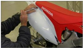
3. Remove lower OEM muffler mounting bolt. Retain for use.
