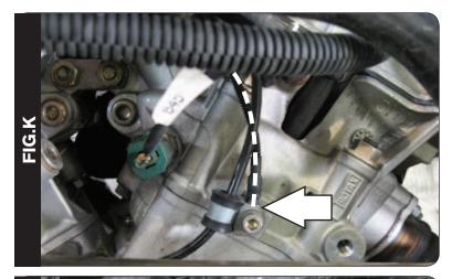
17 Attach the ground wire of the Juicebox Pro to the rear cylinder head on the left side (Fig. K).
