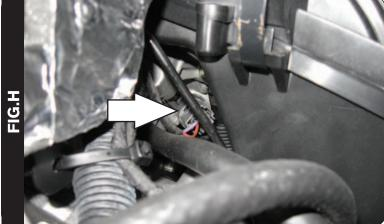
13 Unplug the stock wiring harness from the injector on the right hand side (Fig. H).
