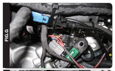
12 Plug the YELLOW colored wires from the Juicebox Pro in-line of the stock wiring harness and injector.
