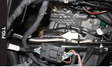
18 Unplug the stock wiring harness from the front O2 sensor (Fig. L).
