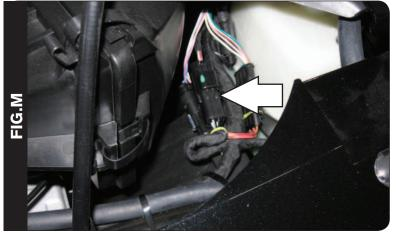
20 Unplug the stock wiring harness from the rear O2 sensor (Fig. M).
