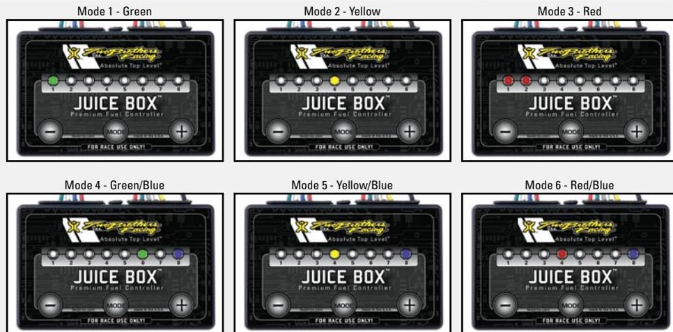
**Additional Setting:** YFZ450R with airbox lid OFF, TBR FULL exhaust with spark arrestor (G=0.5, Y=4, R=1.5, GB=6, YB=4, RB=4)
