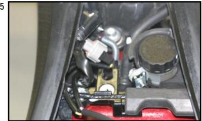
5. Route wires to rear of ATV and secure the JUICE BOX™ with the supplied velcro and zip ties to the wires secure to frame.
