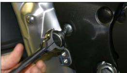
6. Loosen muffler joint clamps
