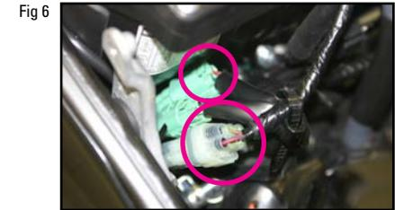
8. Unplug OEM connectors and plug-in the JUICE BOX™ and back into OEM harness as shown. (fig. 7)
