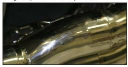
Attach muffler to TBR slip system using the supplied X-ring, 6x14mm socket head cap screws and lock washers that are provided, leave loose for now.
