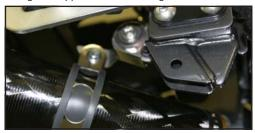
Check for clearance and alignment, then tighten all the bolts in this order: Header flange nuts, X-ring bolts, and then muffler mount bracket.
