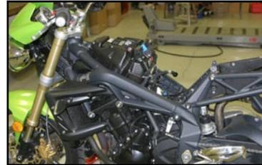
4. Locate the injector and O2 sensor plugs. Unplug one at a time and plug the male/female ends into the JUICE BOX™ plugs as shown for all the injectors and the O2 sensor.
