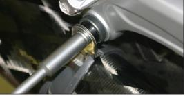
Check alignment of muffler and tighten the 4 6x14mm socket head cap screws. Then tighten barrel clamp and lastly tighten muffler mount.
