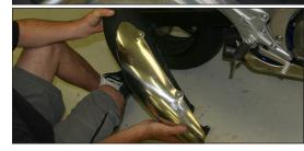
Install TBR muffler to slip-tube shown using the supplied X-Ring and bolts with lock washers, keep loose for now. Loosely Install barrel clamp at end of slip-tube.
