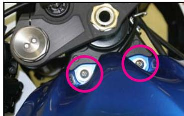
5. Slip the Juice Box between the right fork tube and the steering stem and secure the Juice Box to the sub frame below the LCD display using the supplied adhesive backed hook and loop patch. (Fig. 4)
