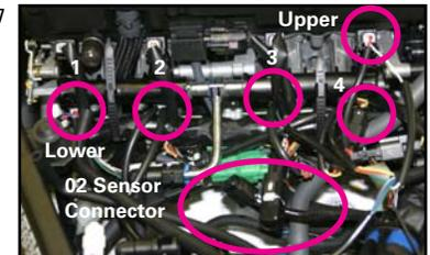
9. Note: Connect the Juice Box connectors with the RED, YELLOW AND WHITE wires to the far right injector (cylinder 4). Connect the GRAY AND GREEN to the right injector (cylinder 3). Connect the BLUE AND RED to the left injector (cylinder 2). Connect the GREEN AND WHITE to the far left injector (cylinder 1).
