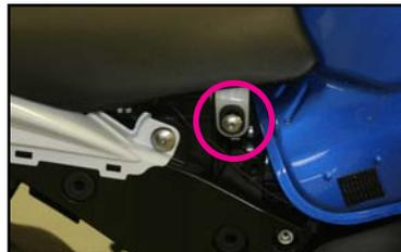
4. Remove bolts (2) that secure the front of the fuel tank to the frame near the steering stem. (Fig. 3) Rotate the tank back and prop up. Alternatively, the tank may be completely removed for better access to the fuel injectors.
