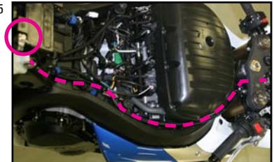
7. Locate the four upper and four lower fuel injectors. Disconnect the upper right injector (cylinder 4) and connect the Juice Box connectors with the SINGLE WHITE wire onto the injector and into the OEM injector connector. (Fig. 6)
