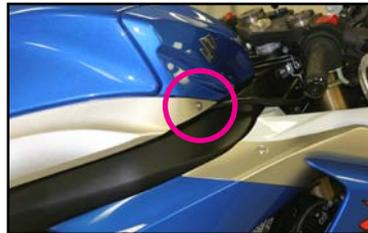
3. Remove bolts (2) that secure the front riders seat. (Fig. 2) Remove the seat.
